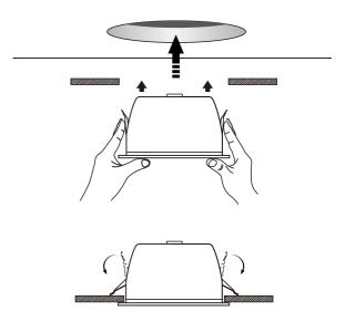
4、 Finally, inspect whether it is installed in a firm and reliable way.
